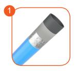
Solid construction made of black steel S235JR, cleaned in the sandblasting process. Protected against corrosion by galvanizing and powder coating with polyester paint QUALICOAT attested. 1 -steel, 2 - sandblasting, 3 - iron phosphatizing, 4 - zinc base, 5 - polyester powder paint.
